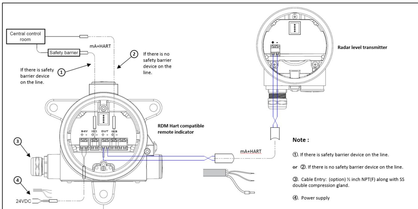
*Remote indicator via Serial communication (LRD-21)*
